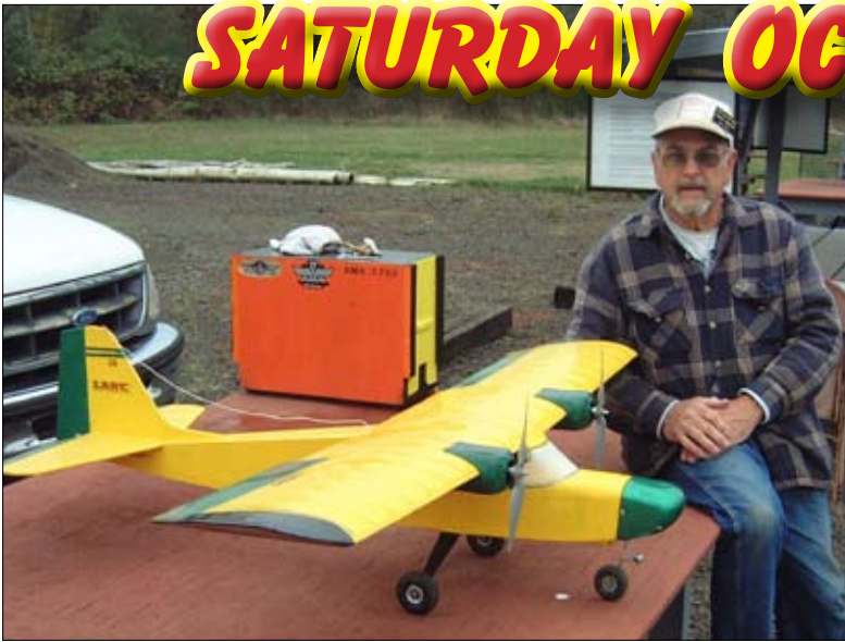
Another of Larry Baker's electric twin engine models. This one is powered with brushed, geared, "can" motors. It has a unique sound in the air. Saturday Oct. 15 was overcast and misty but three of us got in some good flights.
